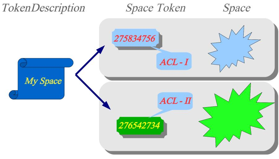
ACL's can only be applied to space tokens, not to space token descriptions, which can lead to unexpected behavior if ACL-Iand ACL-II differ.
