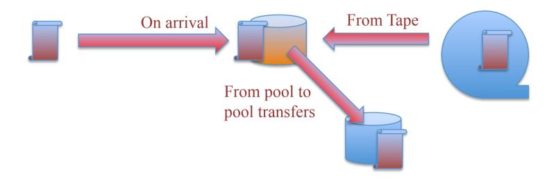
Checksums are calculated on all transfers (except for reading) and if triggered on an entire storage pool.
