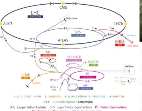
AD Antiproton Decelerator CTF3 Clic Test Facility CNGS Cern Neutrinos to Gran Sasso ISOLDE Isotope Separator OnLine DEvice LEIR Low Energy Ion Ring LINAC LINear ACcelerator n-ToF Neutrons Time Of Flight
